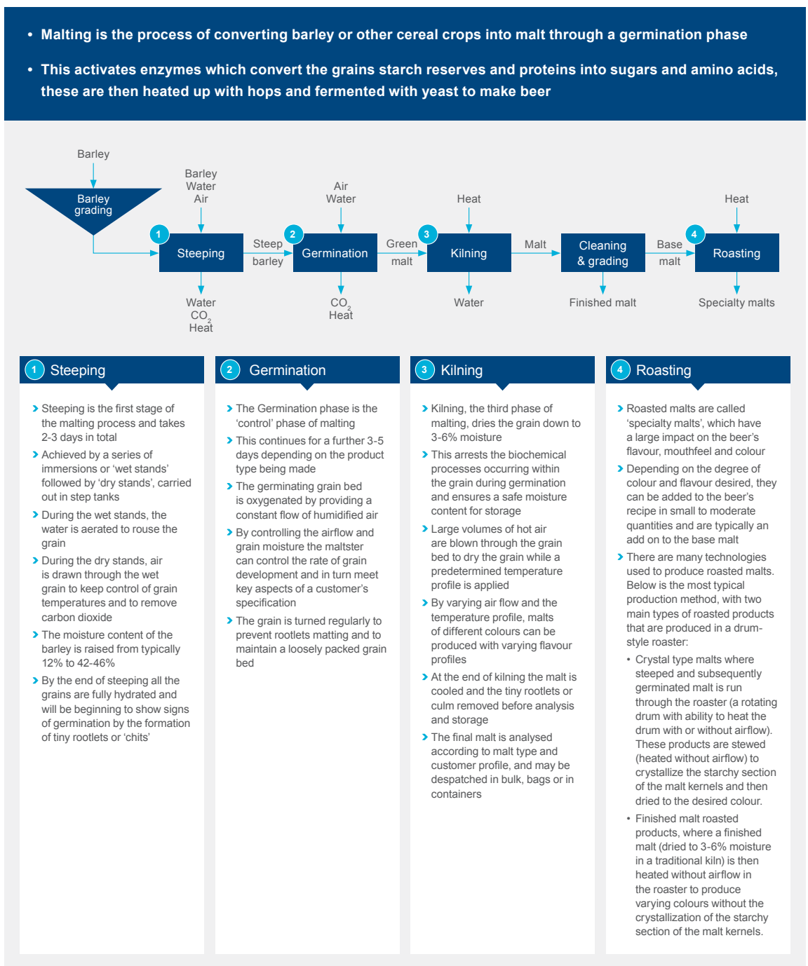
Figure 2.3(a): Overview of the malting process
